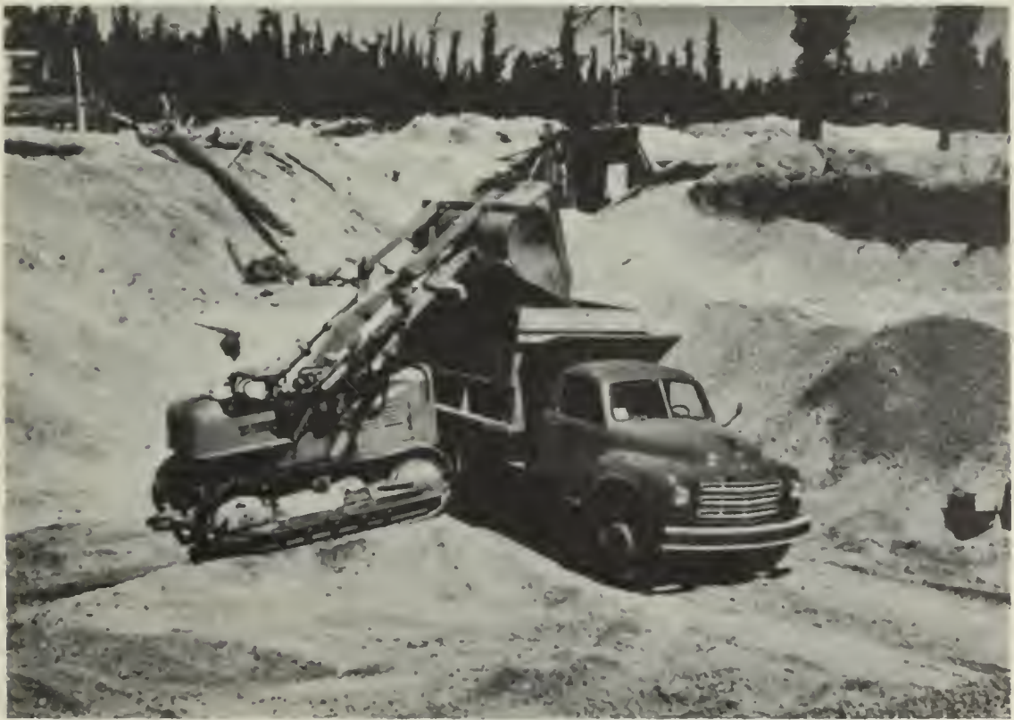
B, FOUCH-THOMPSON PUMICE PIT Siskiyou County. Loading pumice for use as light-weight aggregate in building blocks. Charles W. Chesterman, photography, 1948.
